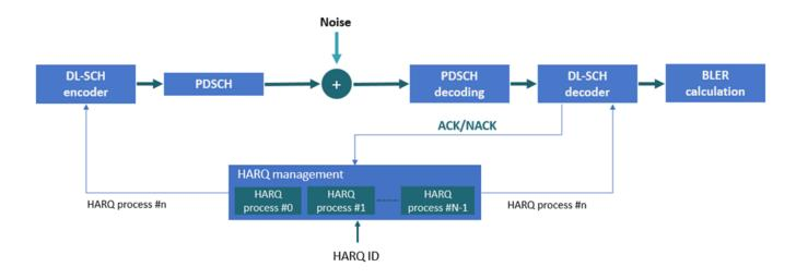
This figure shows that the DL-SCH encoder uses internal buffers to store the transport blocks for each HARQ process and then selects the active HARQ process buffer content for the encoding. The DL-SCH decoder uses a similar buffering mechanism to store and select HARQ processes.
