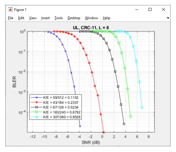
The above results were generated by simulating, for each SNR point, up to 1000 frame errors or a maximum of 100e3 frames, whichever occurred first.
