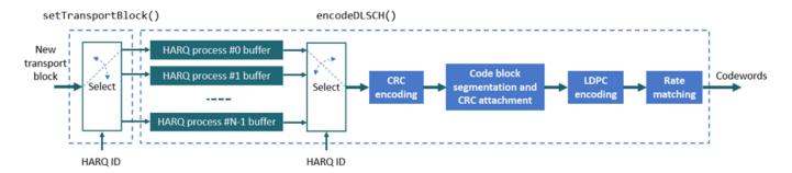
The DL-SCH encoder and decoder do not manage the HARQ processes internally. The example uses the HARQ entity object, HARQEntity.m, for HARQ process management. This figure shows the structure of the HARQ entity object
