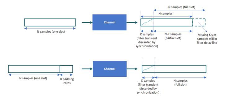
Pad the input signal with enough zeros to ensure that the generated signal is flushed out of the channel filter.
